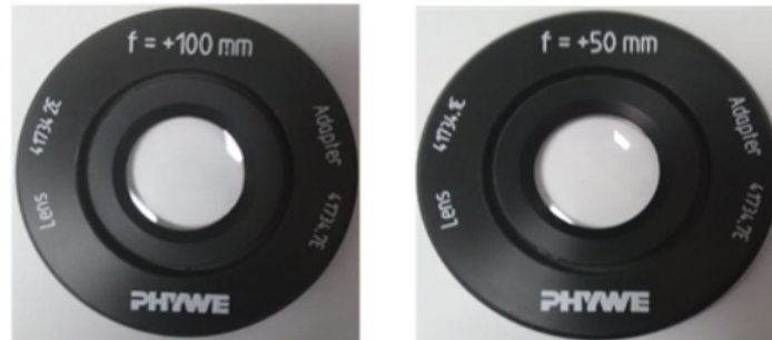
Figure 60 – Lenses used in optical collimation: a lens with f=+100\text{mm} was used for the Transmitter, and a lens with f=+50\text{mm} for the Receiver.
