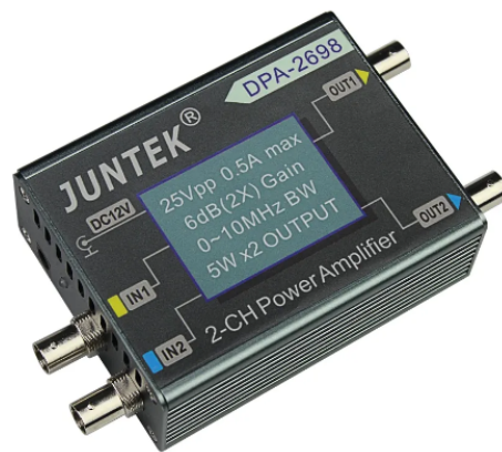
Figure 53 – Juntek DPA-2698 Power amplified employed in the VLC Transmitter
