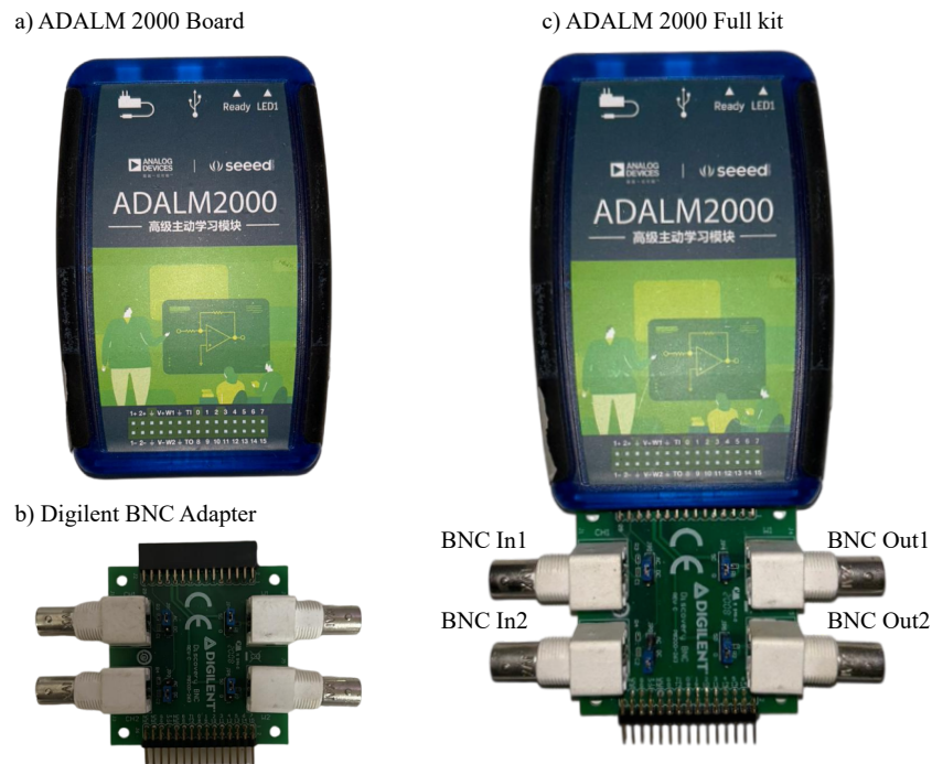
Figure 49 – a) ADALM 2000 Evaluation Board Overview. b) Digilent BNC Adapter Overview. c) Connection between ADALM 2000 and BNC Adapter Board
